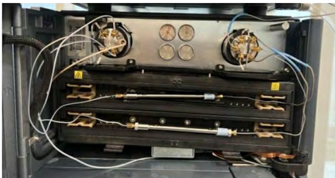
Figure 2. 2D UPLC Hardware Configuration
